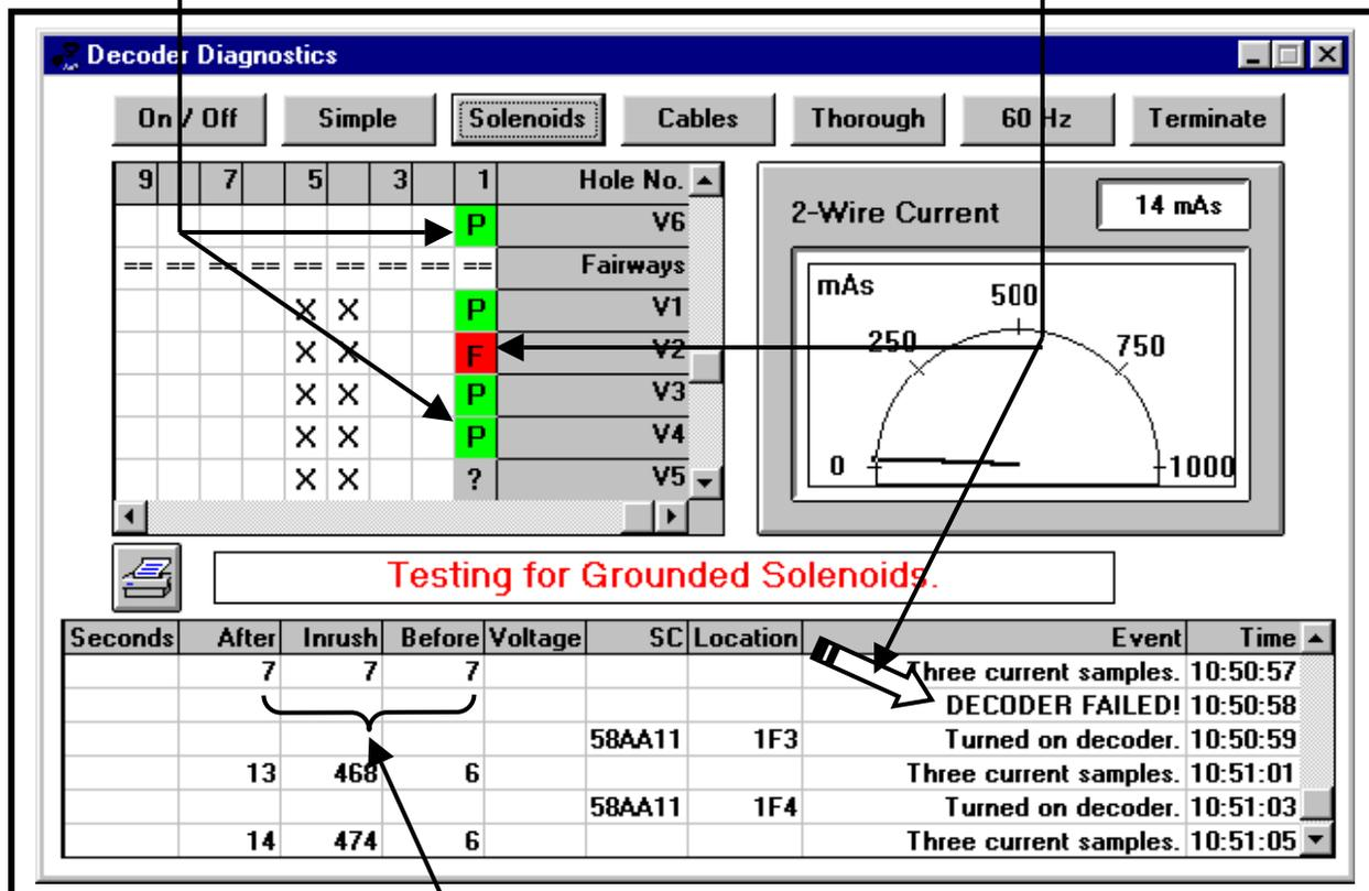
**CURRENTS INDICATE DECODER HAS "FAILED" THIS TEST**
