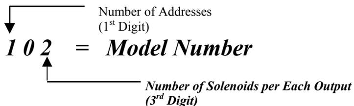
**SENSOR DECODER – Model SD-210:** Can be used either as a “SENSOR” Decoder or as a “PULSE” Decoder. Refer to the “Sensor Decoder” Section immediately following this chart.
