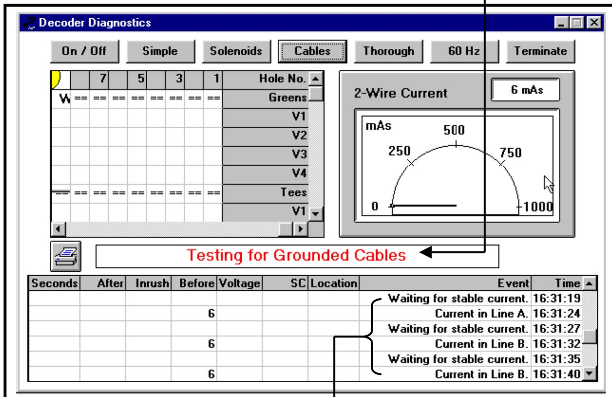
CHECKING CURRENT IN BOTH LINES "A" & "B" OF THE TWO-WIRE PATH
