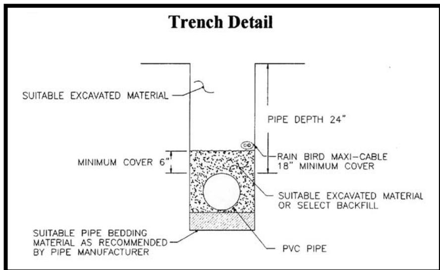
Where wire passes under roadways, cart paths, walls, or any other paved areas or where it may be attached to the under side of bridges, etc., it shall be installed in a minimum of a 2" size PVC Schedule 80 pipe conduit or a conduit that meets local codes.
