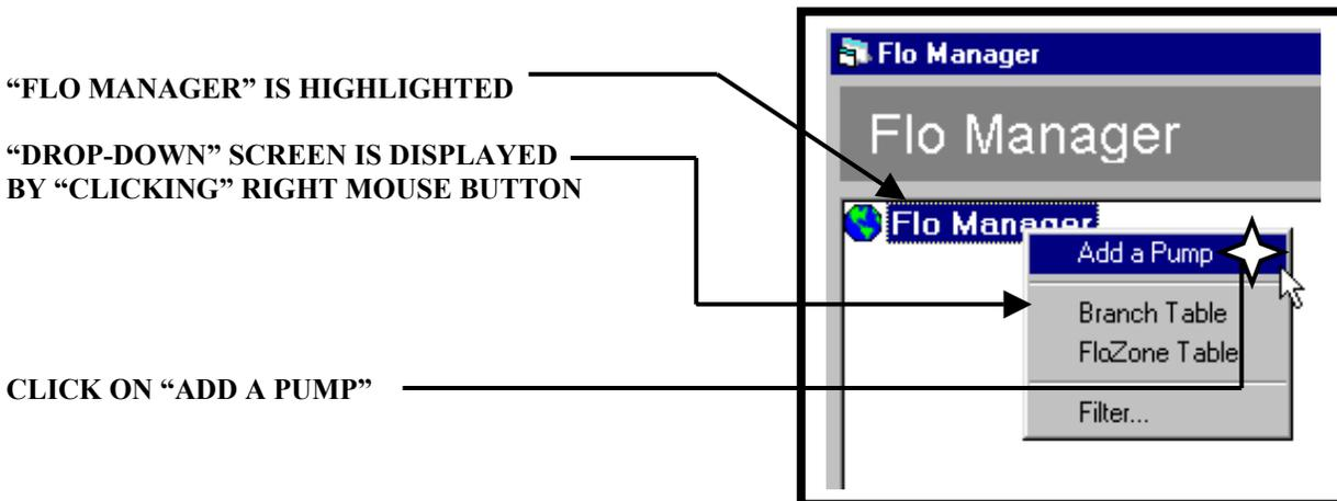
Upon clicking on “Add a Pump” the “PUMP PROPERTIES” screen will be displayed , as shown below.
