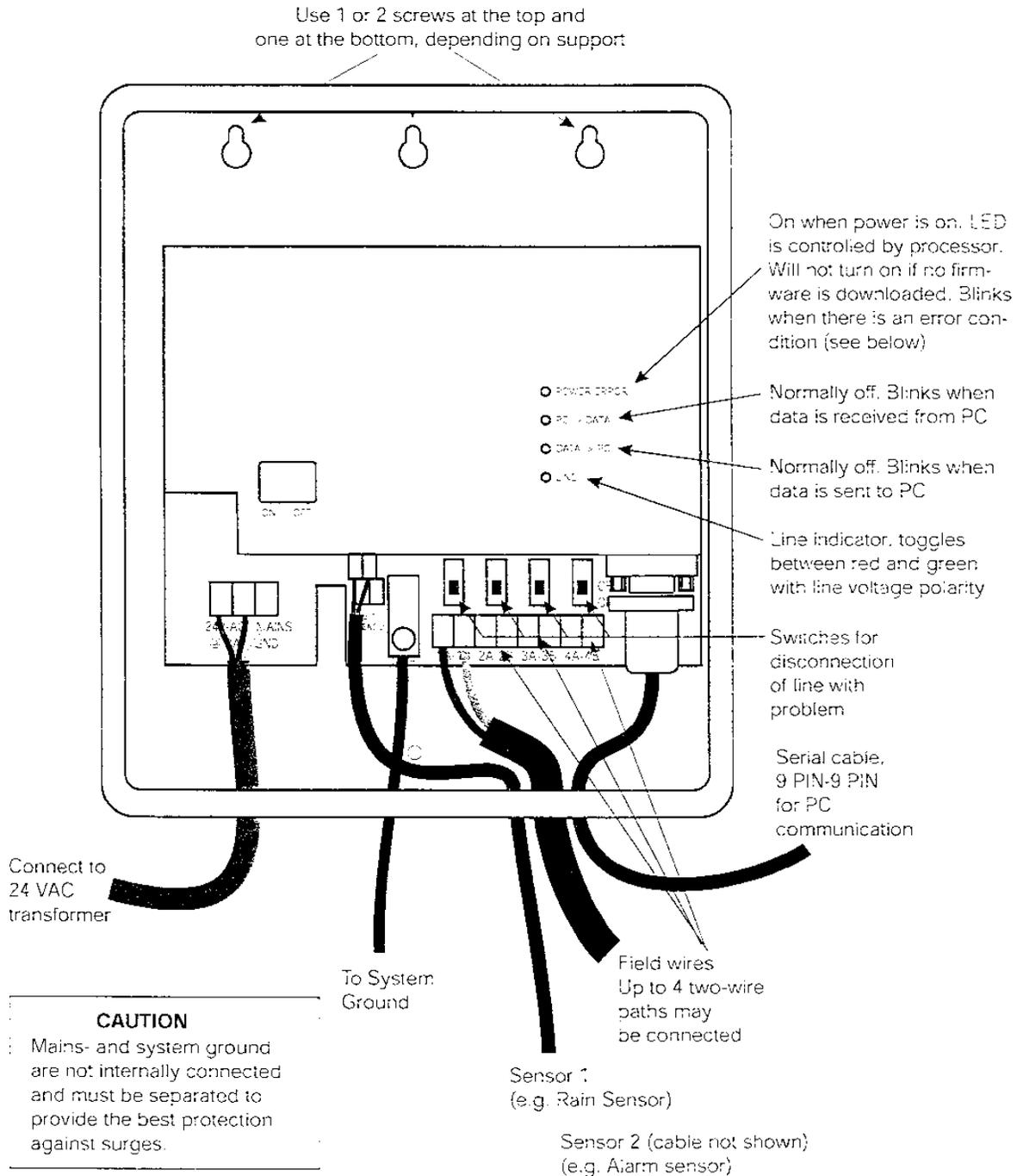
During power up the LED's will blink in sequence ending with POWER LED on for 5 seconds. During those 5 seconds the Flash boot program may be activated for download of new firmware (see special instruction).
