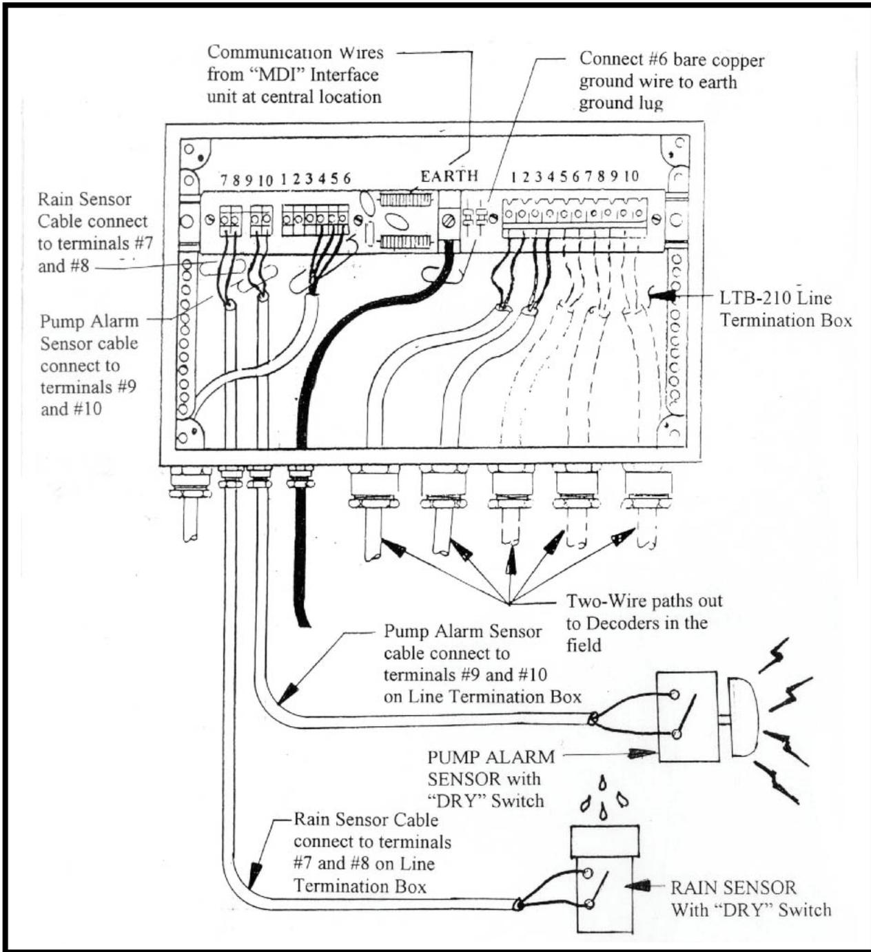
**SENSOR CONNECTIONS TO LINE TERMINATION BOX**
