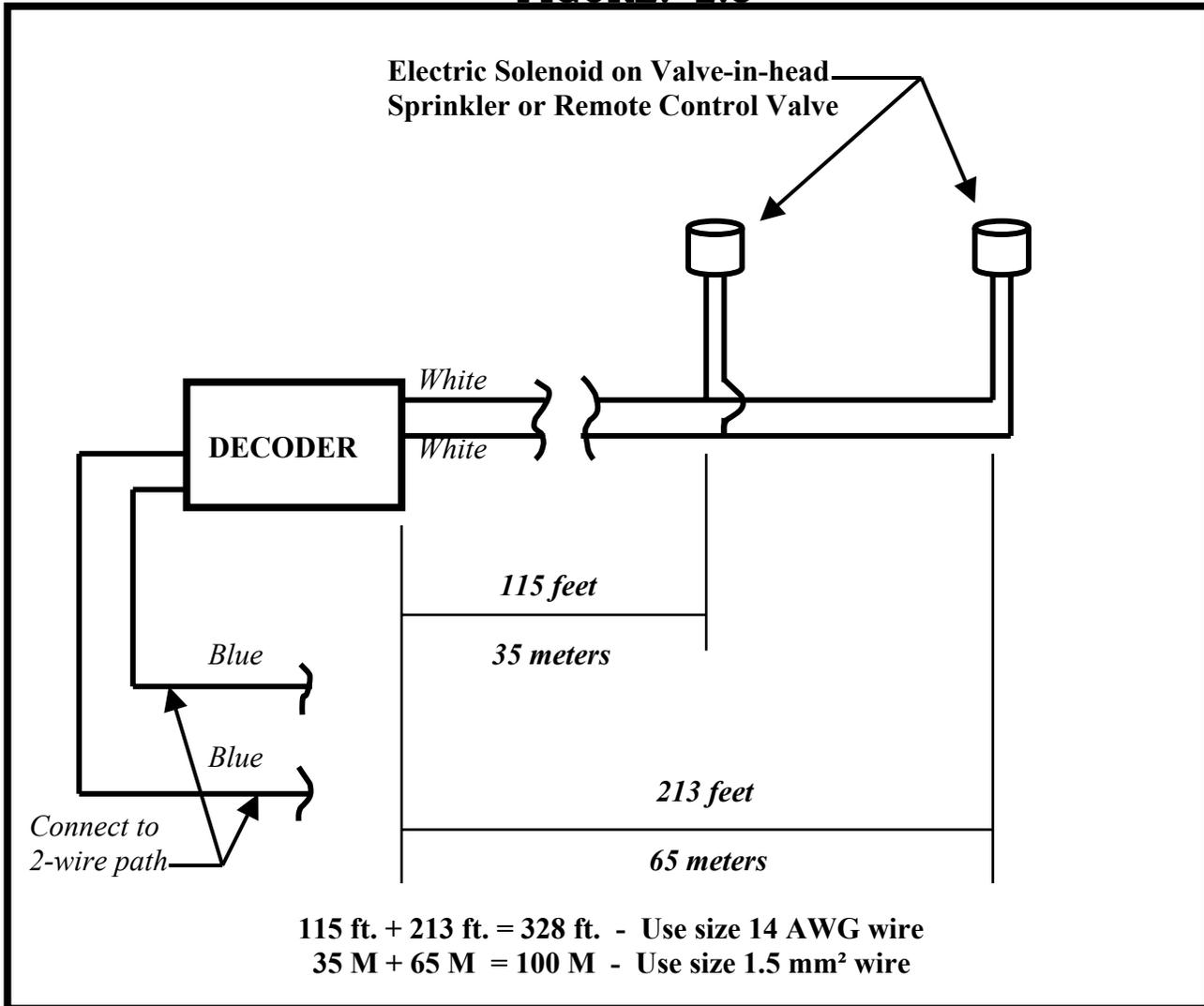
The maximum total length of the secondary wire path, when two (2) solenoids are connected to the decoder output, is defined as the sum of the wire path distance from the decoder to the first solenoid *plus* the wire path distance again from the decoder out to the second solenoid. This means that the section of the wire path that is powering both of the solenoids (the 115 feet/35 meter length in Figure: 2.6) is counted twice.
