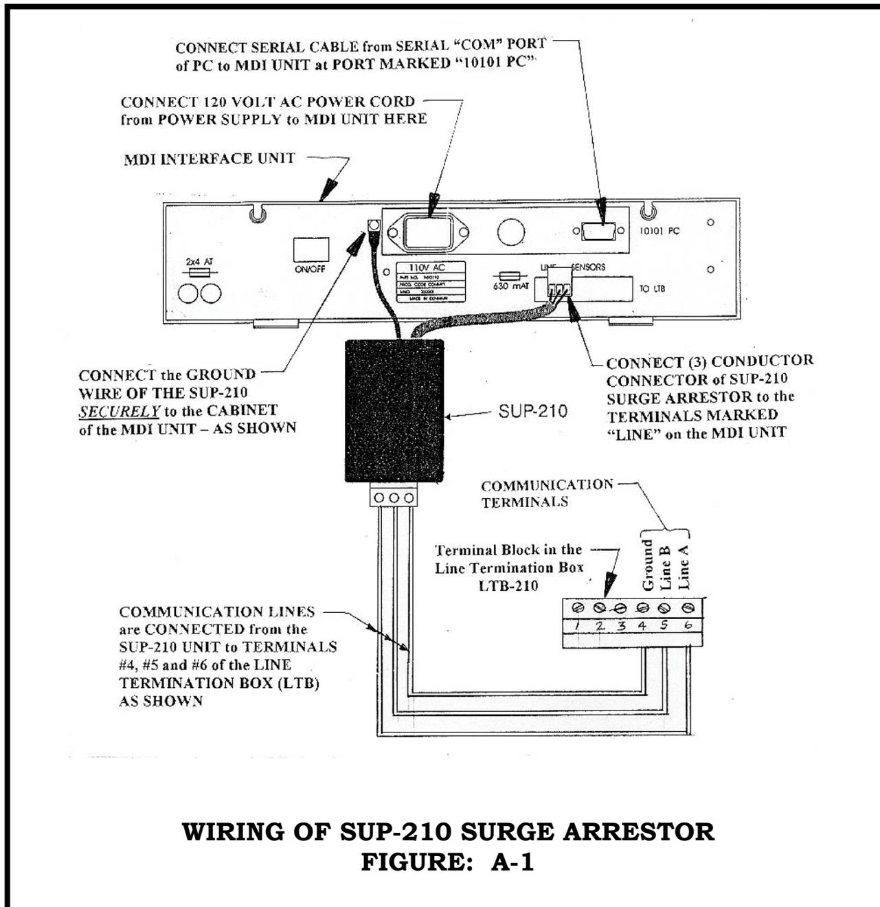
**Communication and Sensor Wiring Between
