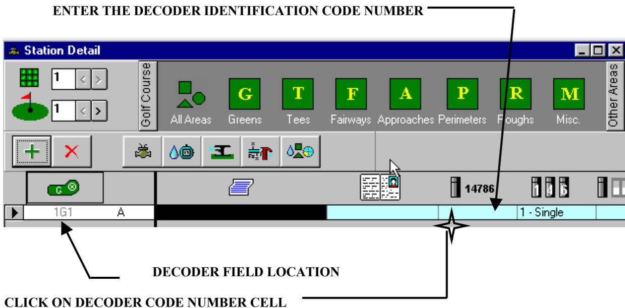
After **CLICKING** on the cell – **ENTER** the Decoder Code Number. In this example use Code Number **1150**.
