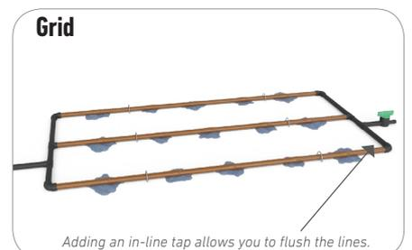
**TIP:** Flush the Drip Eze before 1<sup>st</sup> use to clear any debris that may have entered the tube during installation.
