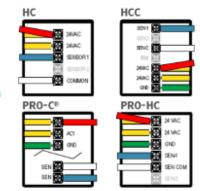
Test the flow sensor connections by turning controller power ON. The LED on the sensor should blink three times on start up to indicate its circuit is active. If it does not blink, disconnect power and connect the red lead to the other 24V power terminal and retry.
