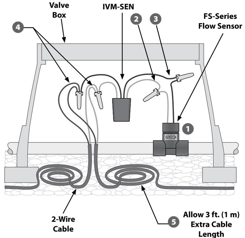
Typical IVM-SEN Flow Sensor Wiring
