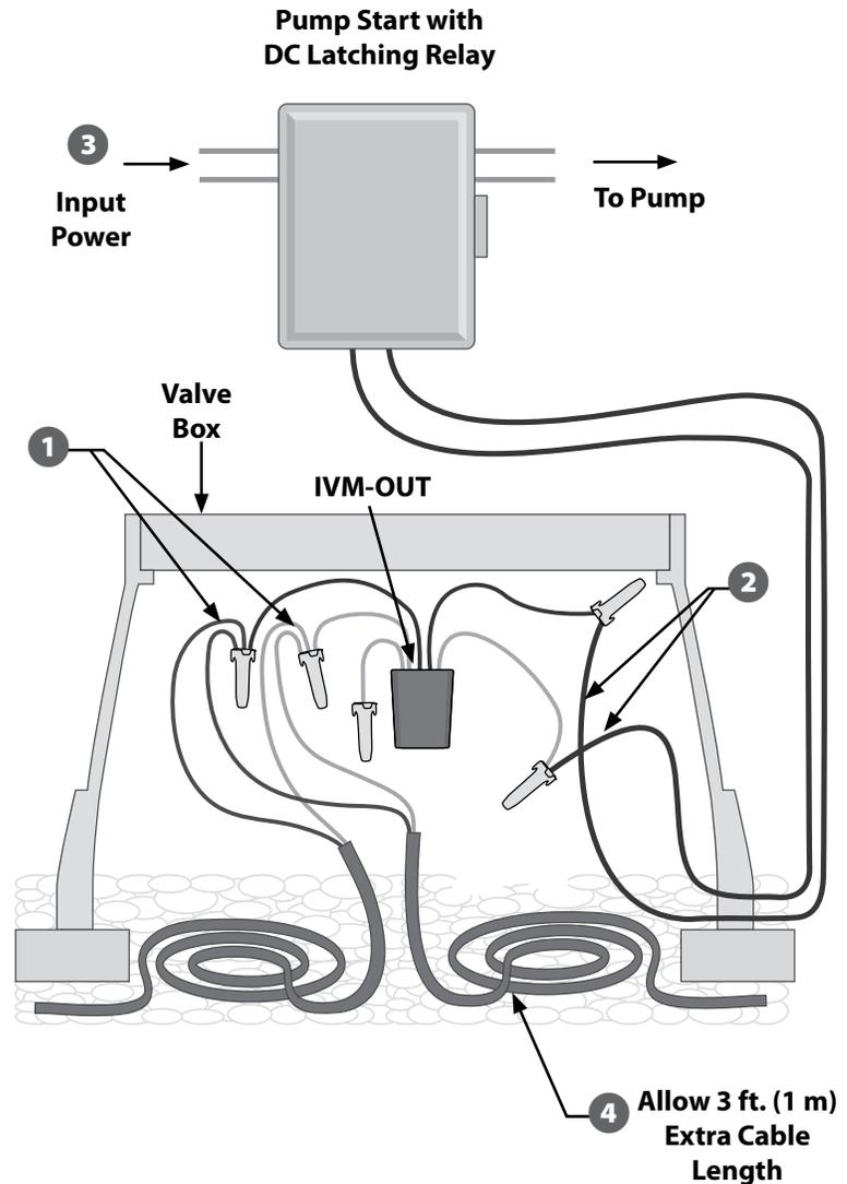
**Typical IVM-OUT Pump Start Relay Wiring**
