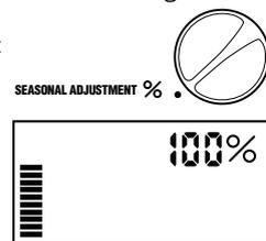
adjust the percentage of the seasonal adjustment. Each bar on the graph represents 10%. This feature can adjust the controller from 10% to 150% of the original program.
