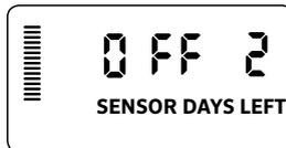
An active Click Delay can be cancelled by turning the dial to the **OFF** position, waiting for OFF to stop flashing, then turning the dial back to the **RUN** position.
