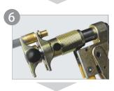
Activate the compression process with either the manual ratchet tool or the hydraulic battery tool until the sleeve reaches the fitting collar.
