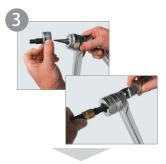
Inspect the expander tool and expander heads prior to use for damage or dirt build up on the heads. Do not use if damaged or missing parts. Ensure the expander head screws completely onto the expander.
