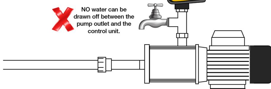
Note: The controller provides dry-run protection in both modes.
