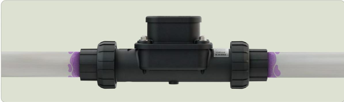
1. Measure and cut a  $7 \frac{3}{16}$ " (183mm) section of pipe to accommodate the FG100, Couplings and PVC fitting. If your installation includes an [in-line valve](#) then you will need to calculate the length of the section to remove based on your components. Make sure the cut is clean, free from burrs, and straight.
