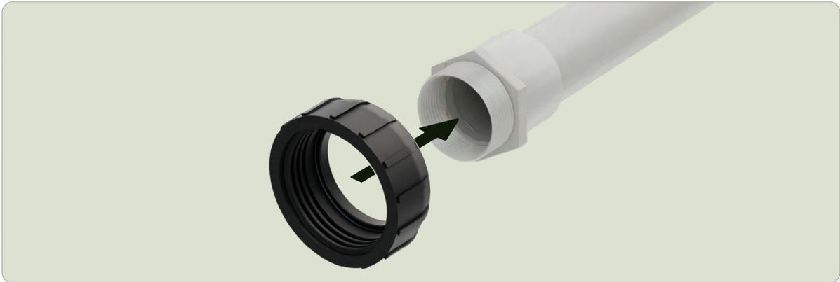
5. Make sure that the pipes are aligned properly to avoid cross-threading. Carefully thread the included NPT/BSP end connector onto the adapters, be careful not to over-tighten.
