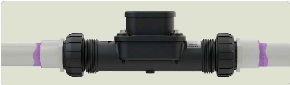
8. Slide the nut over the female end and hand-tighten onto the male end. Avoid over-tightening as this can damage the threads or fitting.
