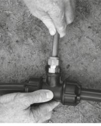
**3. Pipe insertion**Insert the pipe and push it past the olive.
