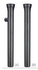
[A] PROS-12-SI [B] **PROS-12** Retracted height: 41 cm Pop-up height: 30 cm Exposed diameter: 5.7 cm Inlet size: 1/2
